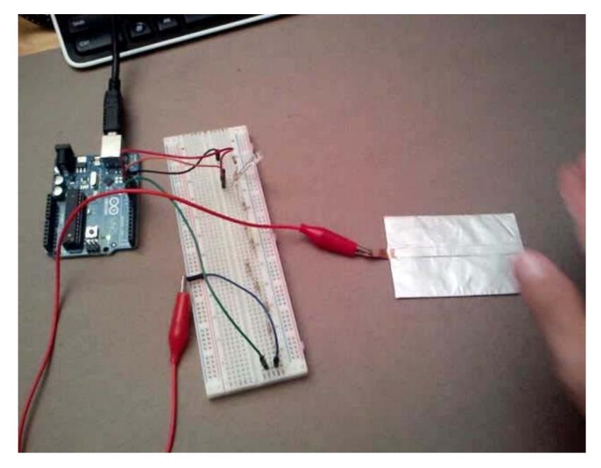
Used sensors :: Felt + conducive film
