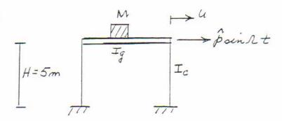
Consider a structural frame having a concentrated mass of 20,000 kg. Assume the girder is "infinitely" stiff in comparison to the columns. Suppose the frame is subjected to a lateral force which is periodic in time, and the design requirement is to limit the lateral displacement to be less than a specified value u\*. Recommend a value for the
