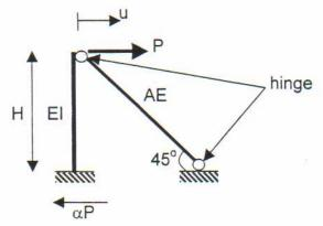
Determine the member stiffnesses such that the shear force in the cantilever beam is equal to  $\alpha P$ .
