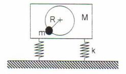
A piece of equipment in the geotechnical lab of the Civil and Environmental Engineering Department at MIT having a mass M of 10,000 kg is to be supported on a foundation. The equipment contains a mass m of 1000 kg rotating at a frequency of 60 rpm and having an eccentricity of R = 0.2m. The force capacity of the floor at the location of the foundation is  $P_{\text{max}}$ =800N. Recommend a value for the stiffness of the foundation.
