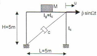
Consider a structural frame having a concentrated mass of 20,000 kg. Suppose the frame is subjected to a lateral force which is periodic in time, and the design requirement is to limit the lateral displacement to be less than a specified value u\*. Recommend a value for the column moment of inertia for the following loading and response criteria. Assume the material is steel.
