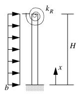
Consider a cantilever beam with a rotational spring at the top. Determine expressions for the shear and bending rigidity distributions corresponding to constant shear and bending deformations.
