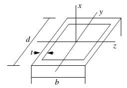
Consider a beam with a closed rectangular cross-section of constant thickness, t.
