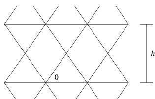
Suppose, instead of plates, the four planes contain diagrids having the geometry shown in the sketch. Estimate the equivalent shear and bending rigidities provided by this bracing scheme.
