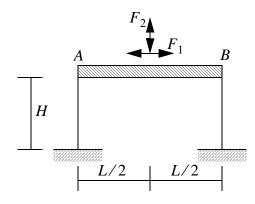
Assume member AB is infinitely stiff. A rotating machine located at mid-span generates horizontal and vertical periodic forces  $F_1$  and  $F_2$ .
