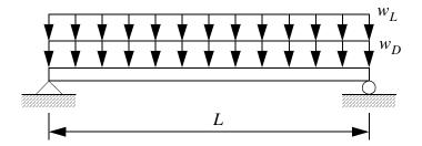
Consider a simply supported beam subjected to 2 uniform loadings,  $w_D$  and  $w_L$ . Strength based design works with the total loading and selects the cross-sectional moment of inertia such that the maximum stress is less than an allowable value,  $\sigma^*$ . Motion based design selects the moment of inertia such that the maximum displacement is less than the allowable value,  $u^*$ . The design code for bridges works with the live load,  $w_L$ , and requires
