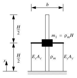
a) Consider a cantilever beam having the mass distribution indicated, no rotational inertia, and an outrigger system. Assuming the beam acts as a bending beam, determine the rigidity distribution required in order for the fundamental mode shape to have the following form:
