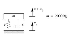
A machine represented by the mass m is to be supported by the spring and dashpot as shown. The machine is sensitive to total acceleration and therefore needs to be isolated from the ground motion.
