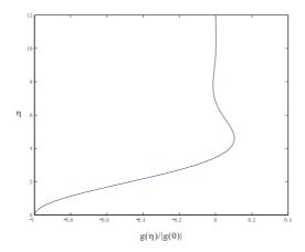
Velocity profile of a 2D slow flow into a line sink in a density-stratified fluid. Calculations by G. D. Lee, 2002
