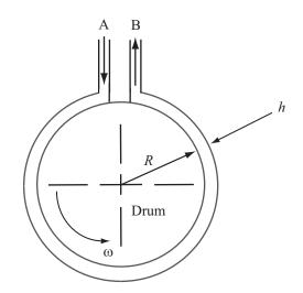
(a) Find the power delivered to the drum by the fluid and the flow rate, as functions of the pressure drop.
