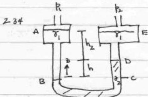
Since  $A_e \ll d_r$ , we assume that the fluid heights open to the air are at the same level, i.e.  $h_A = h_E = h + h_2$ . Compute the pressure at the points A, B, C, D, E:
