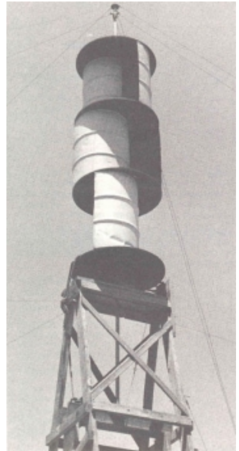
Figure 2-3: Crude Savonius rotor constructed from old barrels. From Park 1981
