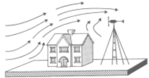
Figure 1a. The house is diverting the wind stream above the generator, which should either be raised or moved.
