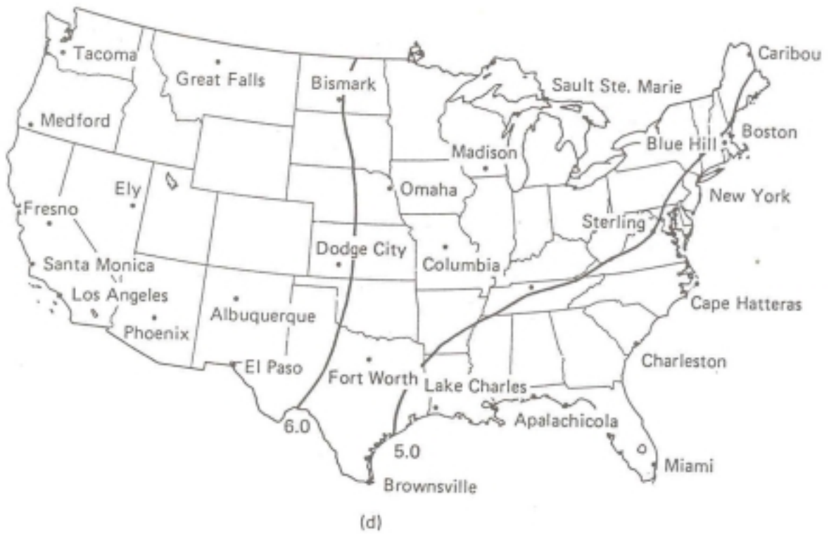
Figure B-2c(d): Average daily availability of total solar radiation on a south-facing 45° tilted surface for the United States in the spring (summer), in kWh/m 2 From Stitt 1999
