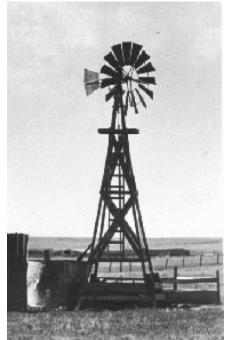
Figure 2-2: Midwest drag machine used for pumping water. From Dodge 2001
