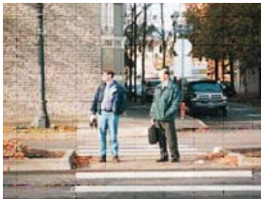
Figure 15: Traffic calming techniques: median is sufficiently wide to allow pedestrians to wait before crossing
