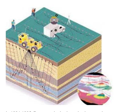
you can also see any changes in the ground versus time. For example shift of layers or flow of material in reservoirs.
