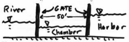
The lock consists of two swinging gates that are 22 feet wide and extend to the river/harbor seabed. No water can "leak" through the locks when they are closed. The two walls are 50 feet apart as shown in the drawing below:
