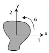
Two dimensional motion with axis (x,y) fixed on the body. 1: Surge, 2: Sway, 6: Yaw
