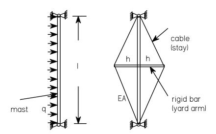
In order to increase the stiffness of the system, the mast is reinforced by four stays (cables), as shown in the sketch above. The stays are held apart by two rigid bars (yard arms) of the length h each. The axial rigidity of the stays is denoted EA. Note that the cables and rigid bars are in the same plane as the distributed load q.
