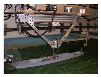
**Lab setup**: This lab is performed in the Ocean Engineering towing tank (48-015). The DDG-51 model is mounted to a free moving linear carriage, and rests in the water at its design draft. In the first part of the lab waves are generated by wave paddle at one end of the tank and the model is fixed. In the second part of the lab, the model is towed at a forward speed in head seas such that the effects of encounter frequency can be observed.
