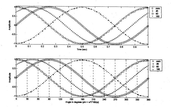
The above plots where generated using Matlab. The upper plot is a 1 Hz cosine function plotted against time, whereas the bottom plot is the same 1 Hz cosine function plotted against the argument angle in degrees.  $(\theta = \omega t)$  Below is the m-file code that was used to generate the plots.
