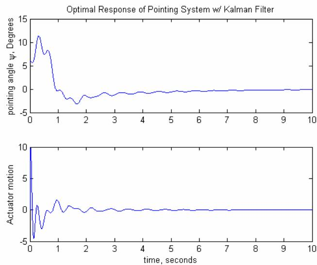
Kalman filter estimator response for the initial state defined above, but no feedback.
