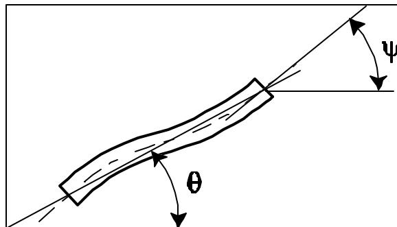
The rigid-body attitude is given by  $\mathbf{q}$ , but the angle that the satellite's optical axis is pointing is corrupted by the flexible modes, and is given by  $\mathbf{y}$ .
