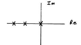
• INCREASING KI TO INCREASE THE SPEED OF THE RESPONSE PUSHES THE POLES TOWARDS THE IMAGINARY AXIS -D OSCILLATORY.
