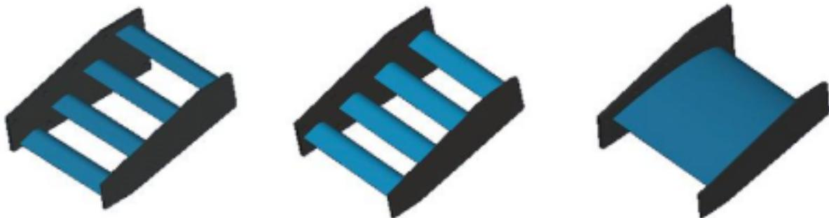
**Figure 8:** From left to right, the finished Equal-Load and Equal-AOA wing grids, and the control tip.
