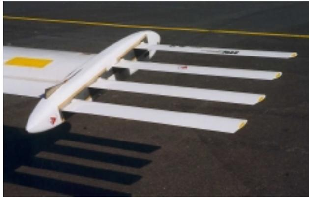
**Figure 1:** A four-winglet wing grid, used for flight testing in France. The four-winglet configuration has been the subject of this project.
