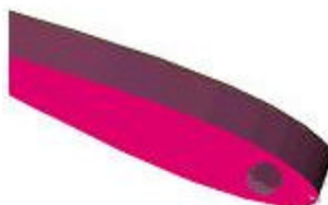
Figure 7: A space for the spar was drilled into the foam.
