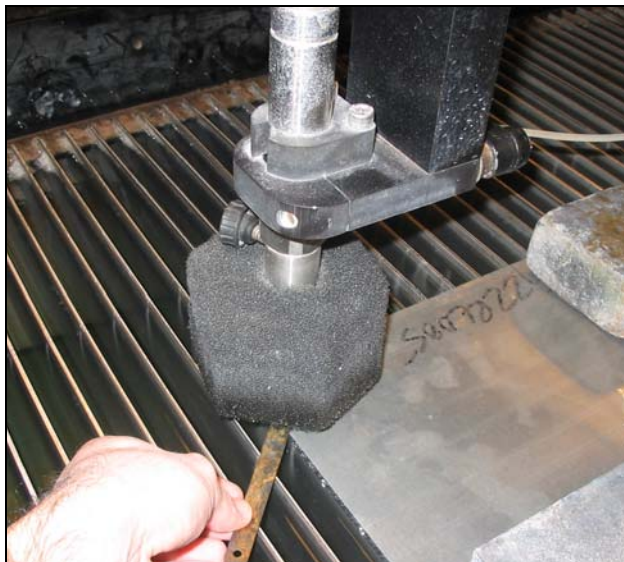
Figure 43 Positioning the height of the water jet cutter nozzle
