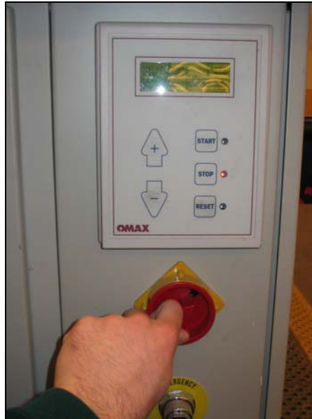
Figure 35 Turning on/off power to water jet cutter
