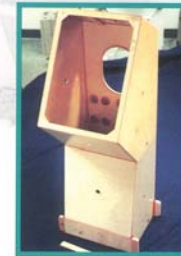
Grapple Mount for Spartan 207/IAE 18" x 15" x 48" x .125 Wall Thickness. Successfully Rawn May 1996.
