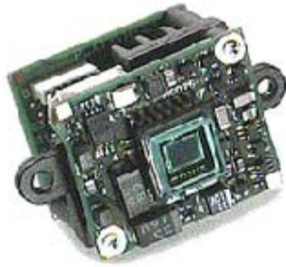
Figure 4.5: Panasonic GP-CX171 CCD board camera without lens or lens mount
