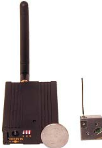
Figure 4.6: 2.4 GHz, 5mW transmitter & receiver set from Black Widow AV
