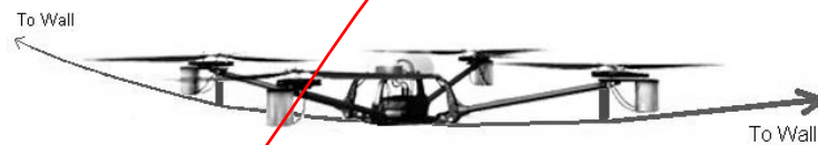
Figure 5.3: Pitch/Roll Controller Test Setup
