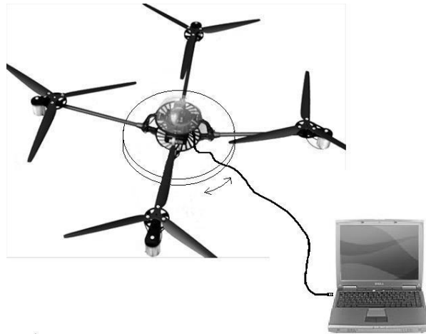
Figure 5.1 Yaw Controller Test Setup
