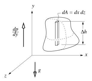
where dp/dy has been replaced by  $-\rho g$  using the Hydrostatic Equation (1), and the volume of the infinitesimal volume is  $\Delta h dA = dV$ . Integrating the last equation above then gives the total buoyancy force on the object.
