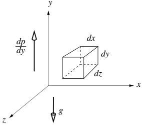
If the fluid element is at rest, the net force on it must be zero. For the vertical y-force in particular, we have
