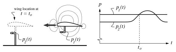
Note that although the two sensors measure the same instantaneous static pressure at the same point (at time  $t = t_o$ ), the measured <u>time rates</u> are different.
