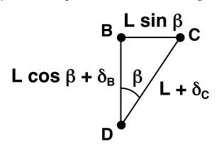
The base assumption is that the angle  $\beta$  does not change. By trigonometric relationships we get:
