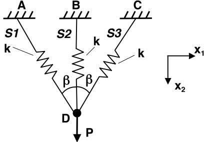
A key factor in considering this configuration is the reality and principle of *symmetry*. This configuration is geometrically symmetric about the BD line including symmetry of load application. Thus, it must behave the same way on either side of this *line of symmetry*. Therefore, the problem needs to only be considered and solved about one-
