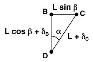
Call the new angle  $\alpha$ . One can note that since the lengths of the springs have increased, the angle will have decreased. From the geometry in this case, we have:
