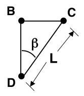
If the length of S3 (from D to C) is L, then the length of S2 (from D to B) is (L  $\cos \beta$ ), and the length along the wall (from B to C) is (L  $\sin \beta$ ).
