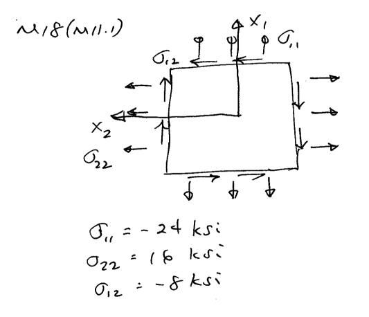
(a) For plane stress the principal stresses are the mots of the equation:  $\tau^{2} - \tau \left( \sigma_{i1} + \sigma_{22} \right) + \left( \sigma_{i1} \sigma_{22} - \sigma_{i2}^{2} \right) = 0$
