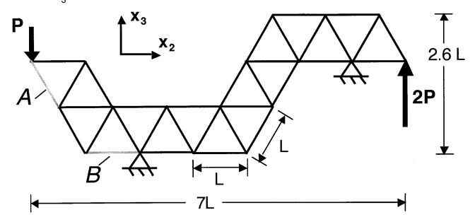
(a) What is the "class/category" of this structural configuration (Dynamic, Statically Determinate, Statically Indeterminate)? Clearly explain your reasoning.
