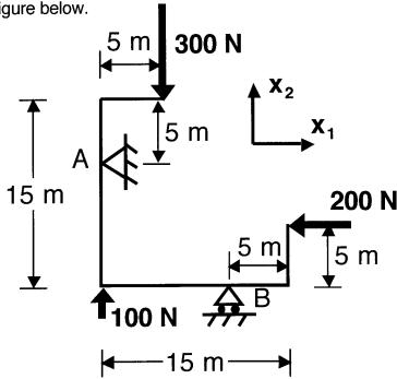
(a) Determine the reaction forces at the two support points A and B *or* indicate all information available to determine the reaction forces and the additional information that is needed to fully determine these forces.
