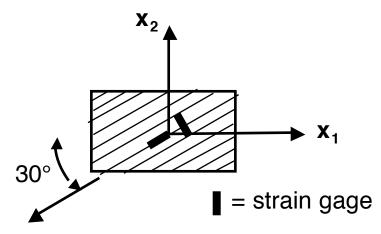
Is it possible to find a transformed axis system in the  $x_1 - x_2$  plane such that the slab is loaded only by normal stresses,  $\sigma_{11}$  and  $\sigma_{22}$ ? If not, describe why not. If yes, describe why, determine the angle to the transformed axis system, and determine the relative values of the normal stresses. **Clearly explain your reasoning.**
