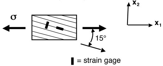
Can the strain readings be determined? If so, do so. If not, clearly explain why not, using equations as appropriate.
