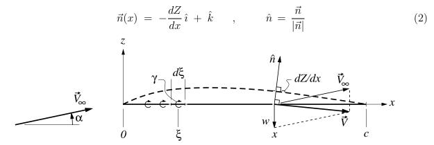
To force the total velocity to be parallel to the camberline, we now apply the flow tangency condition  $\vec{V} \cdot \hat{n} = 0$ . Performing this dot product between (1) and (2), and removing the unnecessary factor  $1/|\vec{n}|$  gives the fundamental equation of thin airfoil theory.
