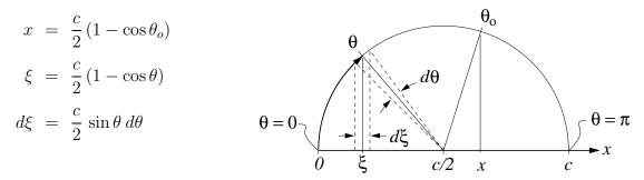
As shown in the figure,  $\theta$  runs from 0 at the leading edge, to  $\pi$  at the trailing edge. Since x and  $\theta$  are interchangable, functions of x can now be treated as functions of  $\theta$ . Equation (3) then becomes
