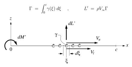
The actual integration of the loading or sheet strength is most easily performed in the trigonometric coordinate  $\theta$ . By direct substitution, we have
