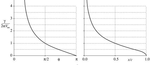
Note that at the trailing edge,  $\gamma = 0$  as required by the Kutta condition, and that at the leading edge  $\gamma \to \infty$ . The latter is of course not physical, although the singularity is weak (integrable), and the integrated results for  $c_{\ell}$  and  $c_m$  are in fact valid.
