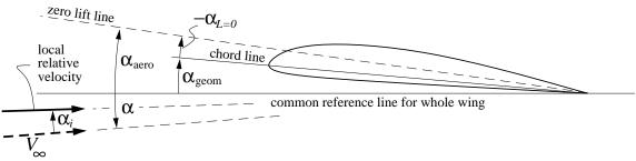
How the geometric twist varies across the span is loosely described by the terms washout and washin:
