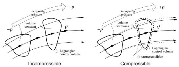
Many of the relations developed for incompressible (i.e. low speed) flows must be revisited and modified. For example, the Bernoulli equation is no longer valid,
