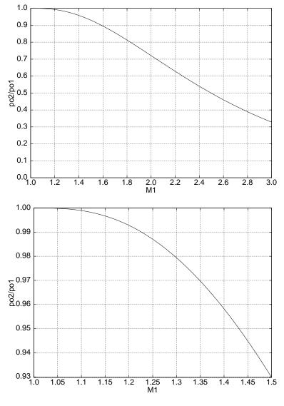
The fractional shock total-pressure loss  $1 - p_{o_2}/p_{o_1}$  is seen to be small for  $M_1$  close to unity, but increases rapidly for higher Mach numbers. Minimizing this loss is of great practical importance, since it cuts directly into the performance of supersonic air-breathing engines.
