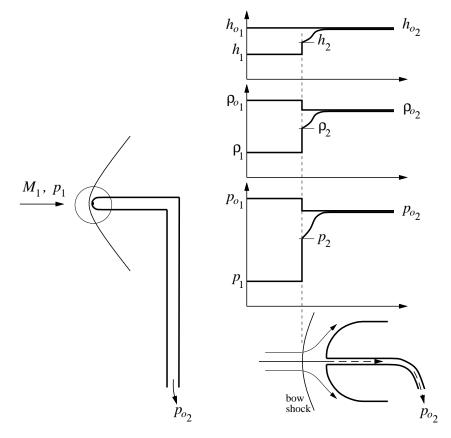
In addition, we also have  $M_2$  and  $p_2/p_1$  as functions of  $M_1$  from the earlier normal-shock analysis. Combining these produces the relation between the  $p_{o_2}$  measured by the pitot probe, the static  $p_1$ , and the required flow Mach number  $M_1$ . After some manipulation, the result is the *Rayleigh Pitot tube formula*.
