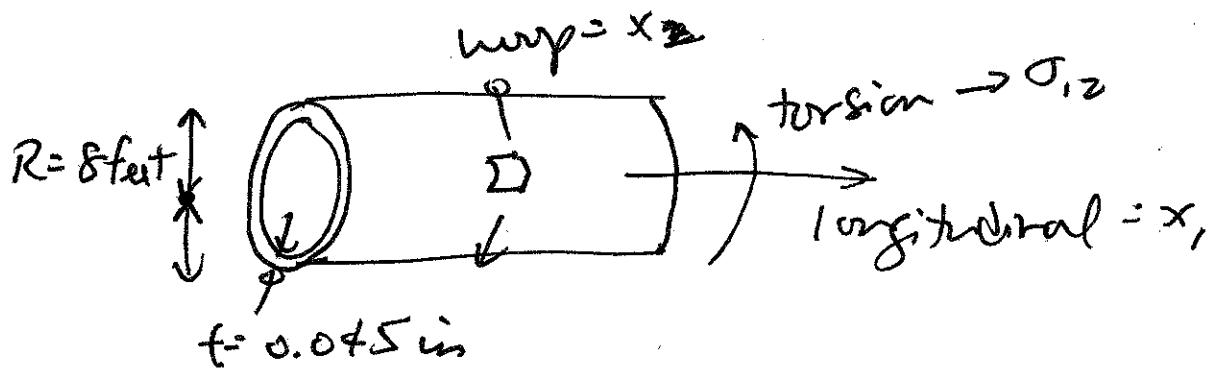
At limit,  $p = 10 \text{ psi}$  (pressure differential)
