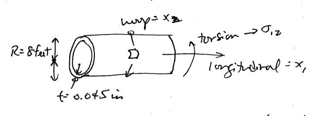
At limit, p=10 psi (pressure differential) pressure dandes or resor of:
