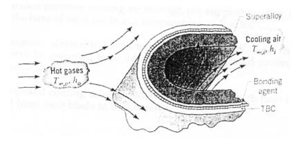
Consider conditions for which hot gases at  $T_{\infty,o} = 1700K$  and cooling air at  $T_{\infty,i} = 400K$  provide outer and inner surface convection coefficients of h<sub>o</sub>=1000 W/m<sup>2</sup>K and h<sub>i</sub>=500 W/m<sup>2</sup>K, respectively. Radiation effects may be neglected, and the turbine blade may be approximated as a plane wall. Let's first assume that TBC is not being used.
