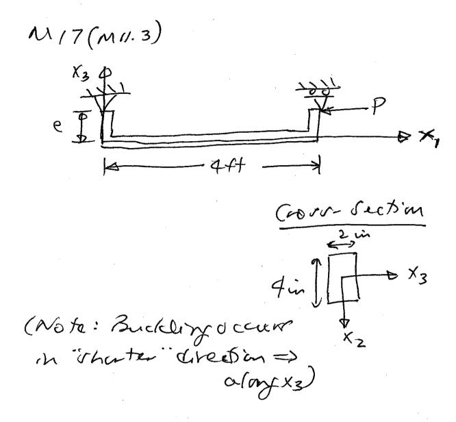
(a) The waxi mum load is the limit placed by the buckling load.
