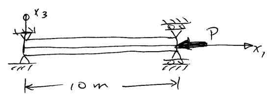
(a) Model this ar a simply-supported column. For a simply-supported configuration:
