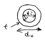
with  $d_i = d_0 - 2t$ fring:  $r_0 = \frac{d_0}{2}$   $r_i = \frac{d_i'}{2} = \frac{d_0}{2} - t$  $= r_0 - t$
