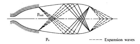
Maximum thrust is for an ideally expanded flow, so although the pressure forces are smaller, the increase in forces due to net momentum flux will outweigh this, leading to increased overall thrust. At the same time the specific impulse will increase, because more thrust will be produced for each unit of propellant flow rate.
