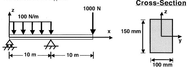
(a) Sketch the shear force and bending moment resultant distributions as a function of position along the beam. Be sure to note the key values of each and their locations.
