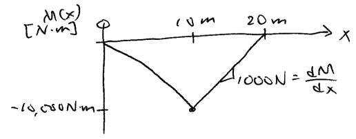
(b) Determine the x-location of the maximum shear stress (i.e.  $\sigma_{xz}$ ).
