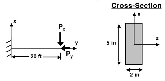
The structural configuration is *subsequently also* subjected to a horizontal tip load along its primary axis,  $P_y$ , of 100,000 pounds.
