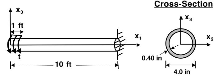
(a) A critical consideration in the design is the rotation of the free end at the critical applied torque. Determine the ratio of that rotation for the two materials being considered.
