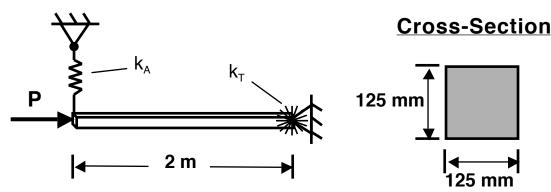
Set up the equation(s) needed to determine the maximum load of this component assuming that manufacturing, alignment, and loading are "perfect". This includes contributions due to *any* deformation prior to instability. Describe how you would use the resulting equation(s) to determine the response but **DO NOT SOLVE**. Use figures if/as appropriate.
