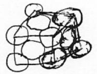
Each unit cell has: B connerveach with "sot the stom when = latom 6 faces each with "2 of an atom in then = 3 atoms To tal = 4 atoms
