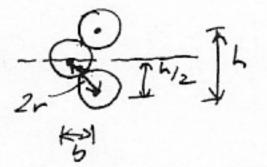
We need the distance "b" from the center of the atom in one plane to the center of the neighbor in the vext plane. Tooking down, we see this atom sits at The midpoint of the equilateral thingh of the first plane:
