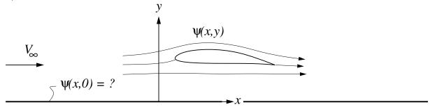
The stream function  $\psi(x, y)$  is to be represented by placing on the airfoil surface a vortex sheet of strength  $\gamma_1(s)$ . At the same time, a sheet of strength  $\gamma_2(s)$  is placed on the fictitious mirror image airfoil of the same shape, as shown.
