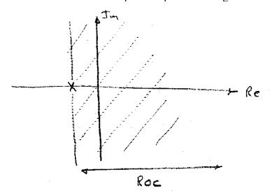
Furthermore, we know that for the Fourier transform of a function to converge then the function must be absolutely integrable. Hence, existence of the Fourier transform is equivalent to system stability. Whence, if the ROC of a system impulse response includes the  $j\omega$  axis then the system is stable. Furthermore, we know that the ROC is always to the right of the right most pole of H(s), Thus, finally, a stable system must have all of its poles in the left half plane.
