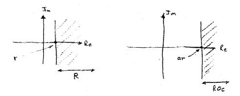
For positive values of a the ROC simply expands or contracts in proportion to a. For negative values of a the ROC is reversed and its size expands or contracts according to the magnitude of a.
