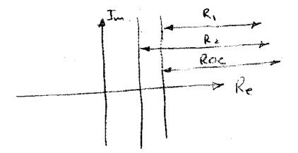
The ROC for a linear combination can be different from the intersection of the two individual ROCs. For example, suppose we have the difference between  $x_1(t)$  and  $x_2(t)$  so
