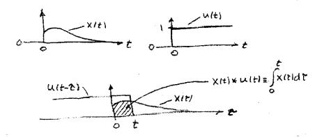
and using the Laplace transform for u(t) and the property that convolution in the time domain implies multiplication in the Laplace domain
