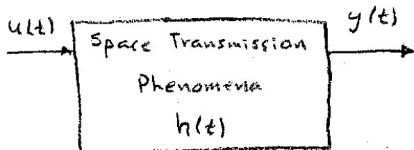
The transmission of the signal through space, from Earth to Moon, has two effects. The signal is attenuated to a very significant amount and it is also delayed in time. Hence the impulse response of the transmission is
