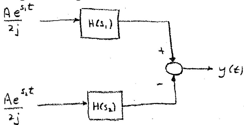
Each of the two input branches is a complex exponential input to the system transfer function so
