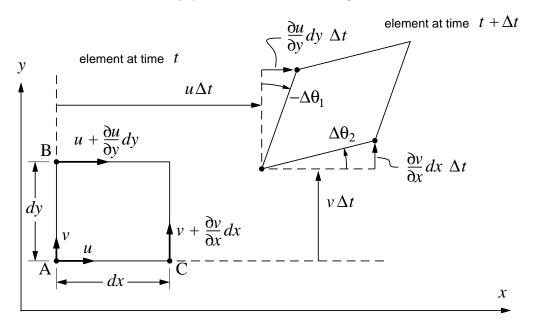
Points A and B have an x-velocity which differs by  $\partial u/\partial y \, dy$ . Over the time interval  $\Delta t$  they will then have a difference in x-displacements equal to
