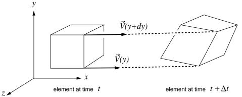
In general, the edges of the element can undergo some combination of *tilting* and *stretching*. For now we will consider only the tilting motions, because this has by far the greatest implications for aerodynamics.
