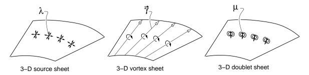
Because  $\vec{\gamma}$  is now a vector, it is not well suited for solution in a panel method. Instead, 3-D panel methods employ doublet sheets, whose doublet strength  $\mu$  (unrelated to viscosity) is a scalar quantity, and can also represent lifting flows. The figure above conceptually shows a doublet sheet. The axis of each infinitesimal doublet is oriented normal to the sheet, rather than along the x-axis as in our previous examples.
