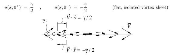
The tangential velocity is then simply a constant  $\gamma/2$  directed clockwise around the sheet. By taking the difference between the upper and lower points at some x location, we obtain a very general tangential-velocity jump condition for any vortex sheet in any situation.
