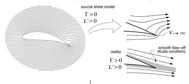
On real airfoils the flow always flows smoothly off the sharp trailing edge, with no large local velocities. This smooth flow-off is known as the *Kutta condition*, and it must be faithfully duplicated in any flow model which seeks to predict the lift correctly. Changing the streamline pattern to force the flow smoothly off the trailing edge requires the addition of circulation, which implies that vortices must be included in the flow representation in some manner.
