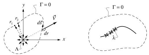
This zero-circulation property of source sheets has severe consequences for flow representation. Any aerodynamic model consisting only of a freestream and superimposed source sheets will have  $\Gamma=0$ , and hence L'=0 as well. Hence, lifting flows cannot be represented by source sheets alone.
