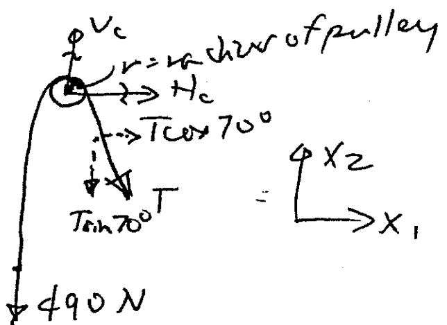
(b) For it to be possible to determine the reactions, the system must be statically determinate (or we need constitutive relations). In this case, that means each of these subsystems must be statically determinate.
