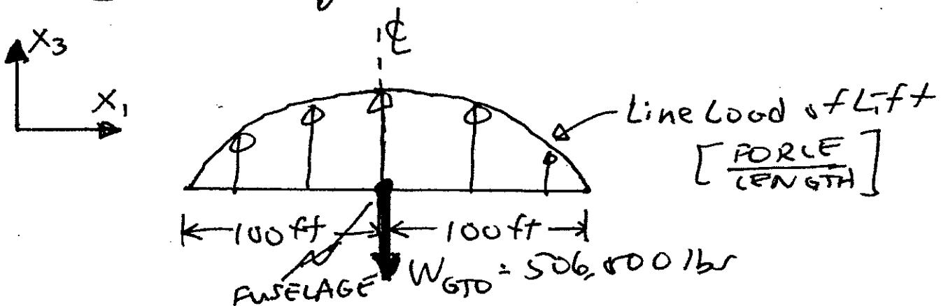
(b) For this we need to consider each lift model and determine values to get an expression for the variation. Place the origin of the  $x_1 - x_3$  system at the root ( $x_1 = 0$ ). Here are the steps.
