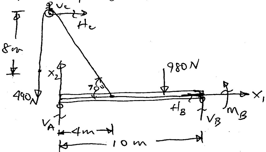
The extra moment reaction,  $M_B$ , is now added to the Beam (sub) system. This adds this term to equilibrium equation (3) ( $\sum M = 0$  for Beam system) giving:
