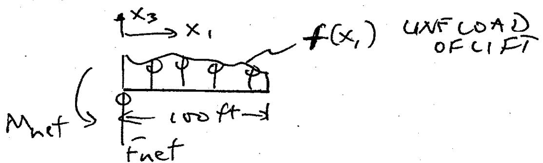
To determine the net force and net moment,  $f(x_i)$  needs to be integrated:
