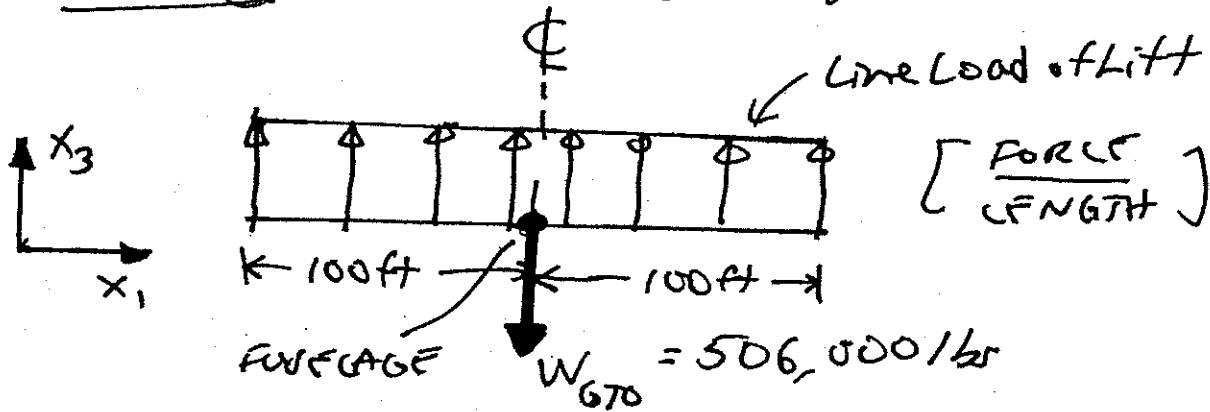
Model ②: linear along span
