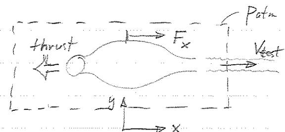
$$\rho V_{test}^2 A_{test} + F_x = 0 \Rightarrow F_x = -\rho V_{test}^2 A_{test}$$
