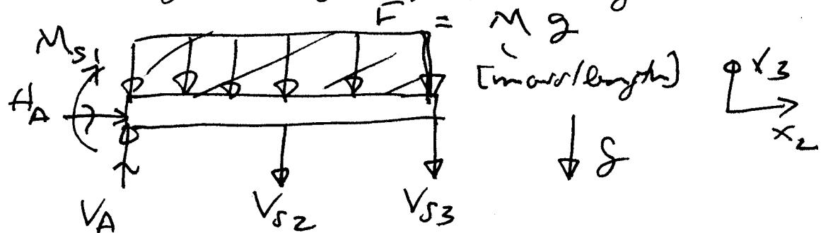
The first spring provides a moment. Springs 2 and 3 provide vertical forces. The force or moments on the bar must be equal and opposite to those on the springs. [Sum to zero for the overall system]
