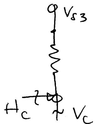
(b) This is a 2-D system and has a potential for 3 degrees of freedom of motion:
