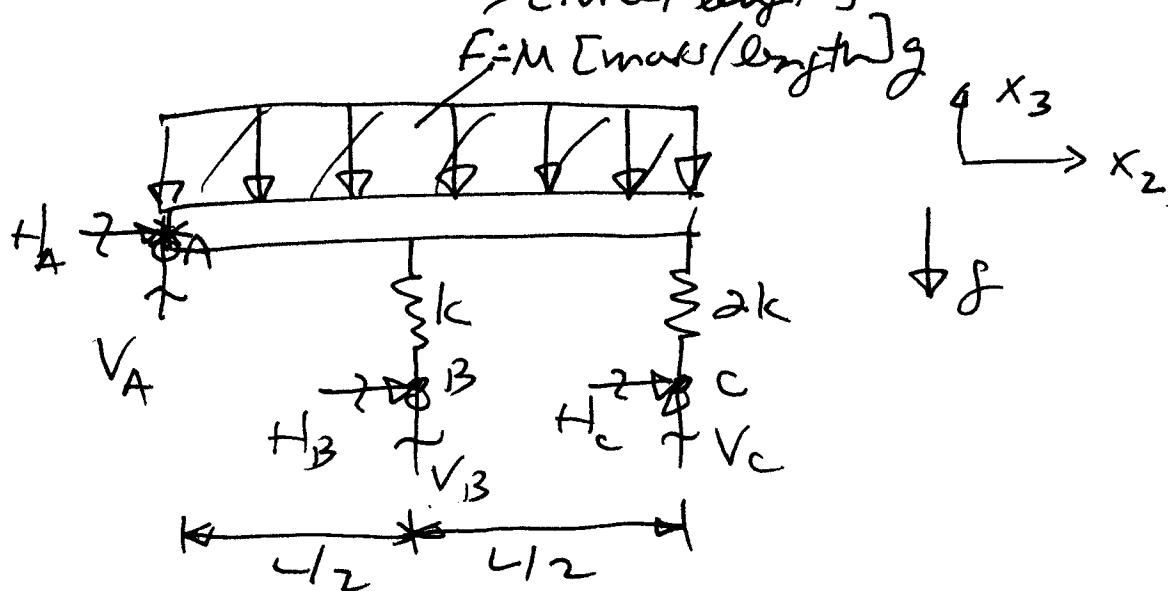
One can look at this as four different subsystems: the bar and each of the three springs acting on it. [Force/length]
