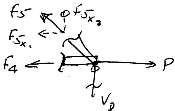
(b) Consider the overall Free Body Diagram of part (a). There are 3 degrees of freedom (in 2-D --- 2 in translation, 1 in rotation) and 5 reaction forces. So there are 3 equations of equilibrium in 5 unknowns.
