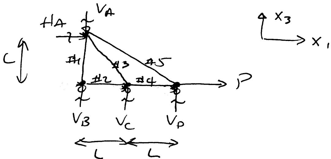
One can also consider each joint as a separate subsystem (Note: This is fundamentally what is done via the Method of Joints):
