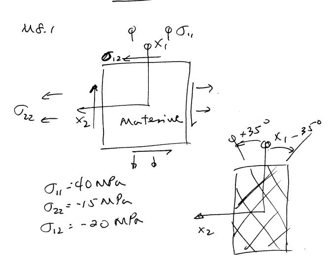
(a) To find the stress state relative to the "fiber axes" align the transformed axis system with its X, axis along the fiber avection. So for the 0 = +35° case:
