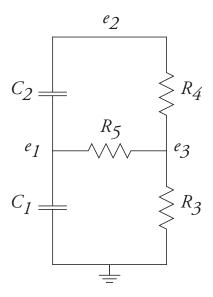
Write down the node equations, using impedances:
