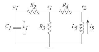
Use the node voltages as labeled above. The node equations are
